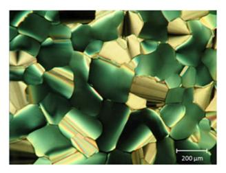
**Figure 4.** LC10 in a confined cell made using glass plates. The sample was cooled down to 120 °C from an elevated temperature at a cooling rate of 0.1 °C/min. The pattern reflects a hexagonal symmetry of the columnar structure with the face-on molecular anchoring.
