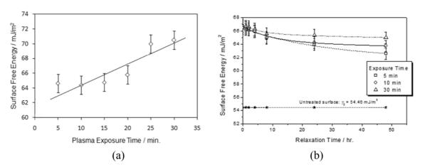
**Figure 5.** Surface free energy of the substrate versus the exposure period of the substrate to plasma.
