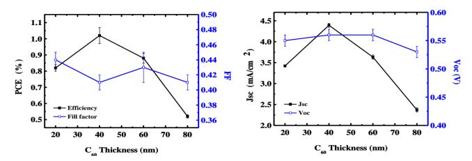
**Figure 5.** Efficiency parameters of OPV devices with different thicknesses of acceptor material. The devices consist of ITO/CuPc  $(20 \text{ nm})/C_{60} \text{ (X)/BCP} (7 \text{ nm})/\text{Ag} (100 \text{ nm}).$
