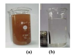
Figure 2. Nanoprobes absorbed before and under the external magnetic field.
