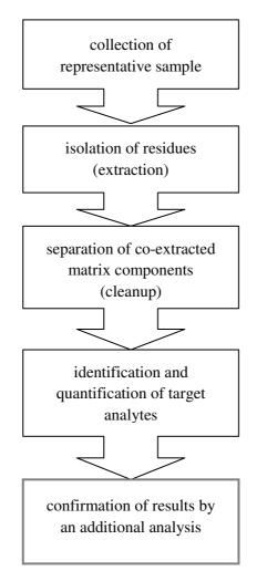
**Figure 1.** Steps in the determination of pesticide residues in samples characterized by complex composition of the matrix.
