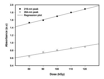
**Figure 9.** Absorption energy of 216 and 264-nm absorption peaks of Pt nanoparticles increased with increasing dose from 80 to 120 kGy owing to a reduction in particle size from 5.3 to 3.4 nm.
