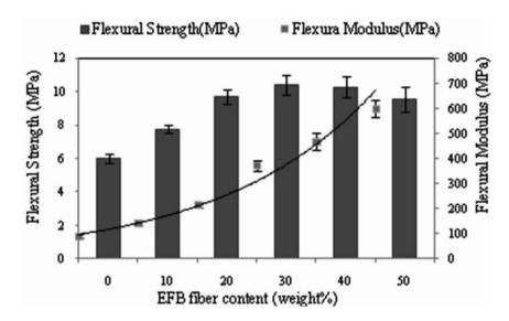
**Figure 4.** Effect of EFB fiber loading on the flexural properties of PBAT biocomposites.
