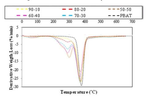
Figure 6. DTG thermograms of PBAT and PBAT/EFB composites in various fiber contents.
