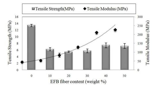
**Figure 3.** Effect of fiber content on tensile properties of PBAT biocomposites.
