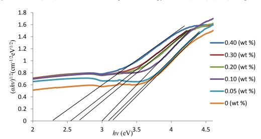
**Figure 3.** The  $(\alpha hv)^{1/2}$  as a function of photon energy, hv for  $(ZnO)_x(SLS)_{1-x}$  glasses.
