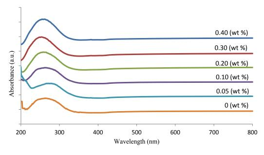
**Figure 2.** Optical absorption spectra of  $(ZnO)_x(SLS)_{1-x}$  glasses.
