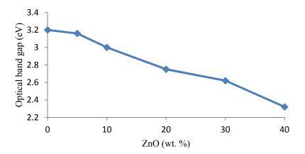
**Figure 4.** The optical band gap  $(ZnO)_x(SLS)_{1-x}$  glasses.
