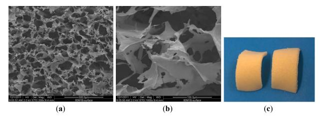
Figure 4a,b are SEM pictures of the of SMC-TCP complex after 60 days of the hydrolytic degradation process, and Figure 4c is a digital picture of sample 60/SMC-TCP.
