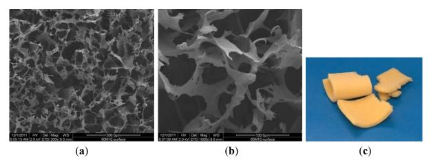
Figure 6. SEM pictures of SMC-TCP complex after 60 days of enzymatic degradation process. (a)  $200\times$ ; (b)  $1000\times$ ; (c) digital picture.
