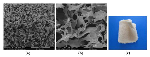
Figure 5a,b are SEM pictures of the SMC after 60 days of the enzymatic degradation (concentration of lysozyme: 200  $\mu$ g/cm<sup>3</sup>) and Figure 5c is a digital picture of sample 60/SMC.
