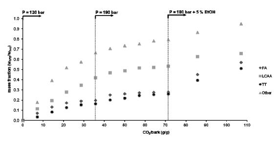
In the first step (120 bar, 40 °C), one extracts mostly long chain aliphatic alcohols and other compounds (41% and 66% of its total potential in the bark, respectively) and low quantities of
