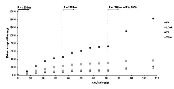
**Figure 6.** Cumulative extraction curves of Figure 5 normalized by the corresponding contents obtained by Soxhlet extraction with dichloromethane taken as reference values. (FA, fatty acids; LCAA, long chain aliphatic alcohols; TT, triterpenoids).
