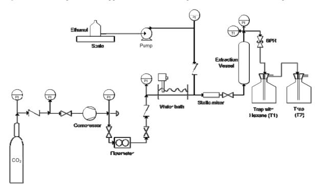
Figure 7. Flow diagram of the apparatus used for the supercritical fluid extraction experiments.
