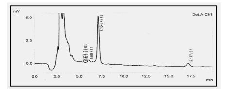
Figure 4. Chromatogram showing high level of AFB1 in gram flour.
