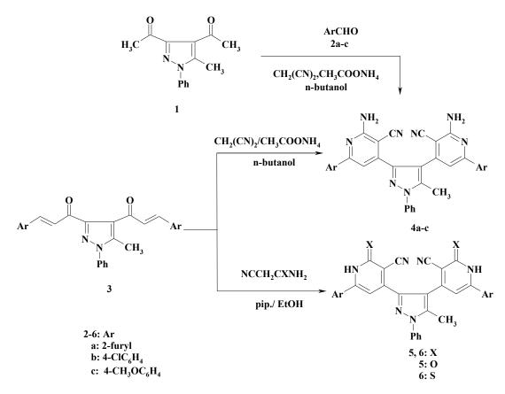
The structures of the newly synthesized compounds were confirmed on the basis of their elemental analysis and IR, <sup>1</sup>HNMR and mass spectral data. The IR spectrum of compound **4b**, taken as a typical example of the series prepared, reveled absorption bands at 2210 and 3438, 3350 cm<sup>-1</sup> corresponding
