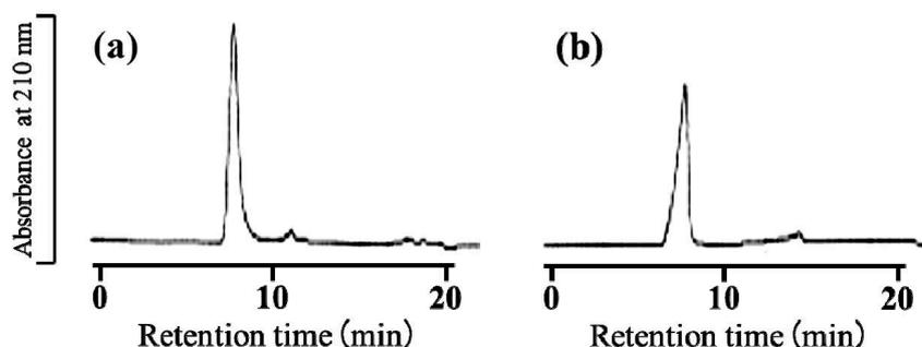
**Figure S1.** Chromatograms in GPC of (a) PGA/HDP and (b) PGA/BZA dissolved in ethanol. Estimated retention volumes (mL): PGA/HDP, 4.9; PGA/BZA, 4.8. The results indicated that both the PGAICs are hydrophobic polymers, the molecular weights of which are on average over 1,000,000 [23,24].
