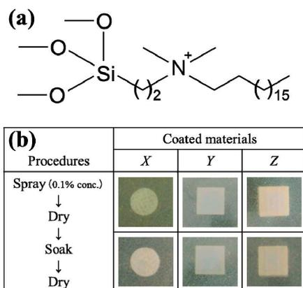
**Figure S5.** (a) Chemical structure of an *n*-octadecyldimethyl [3-(trimethoxysilyl) propyl] ammonium (QAS) cation and (b) anti-staphylococcal activities of QAS-coated materials. Coated materials: images *X*, a PP (*plastic*) disk; *Y*, a stainless steel (*metal*) sheet; *Z*, a bathroom tile (*ceramic*) sheet. The zone of inhibition was not observed around the QAS-coated materials regardless of water-soaking treatment, resulting from its lower anti-staphylococcal activity (Table 2).
