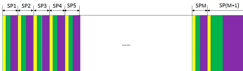
Figure 8. Address display period-separated subfield method (ADS) of DEM for maximum clique problem (MCP). The yellow colors mean the preparation period, the green colors mean the address period, and the purple colors mean the display period.
