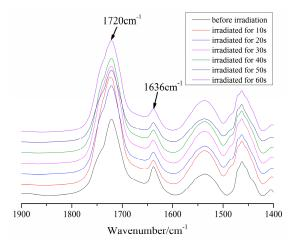
Figure 1. FT-IR spectra during the irradiation process: taking FDMA-based resin as an example.
