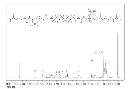
Figure 3. Proton Nuclear Magnetic Resonance (<sup>1</sup>H-NMR) spectrum of FDMA.
