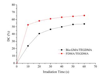
**Figure 4.** The curves of double conversion (DC) versus irradiation time of each dental resin system. Bis-GMA: 2,2-bis[4-(2-hydroxy-3-methacryloy-loxypropyl)-phenyl]propane; TEGDMA: triethyleneglycol dimethacrylate; FDMA: fluorinated dimethacrylate.
