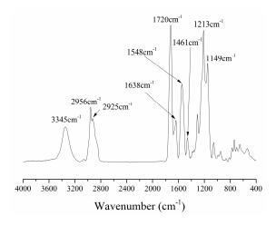
Figure 2. Fourier transform infrared spectroscopy (FT-IR) spectrum of fluorinated dimethacrylate (FDMA).
