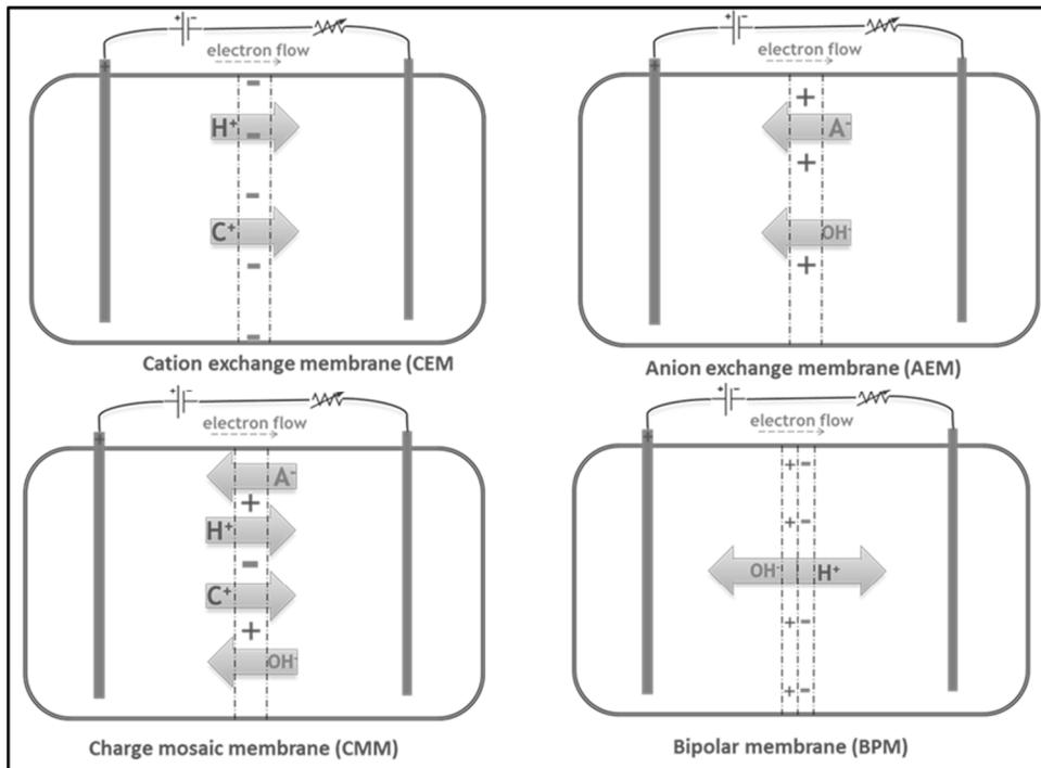
**Figure S3.** Modeling ionic flow across membrane.
