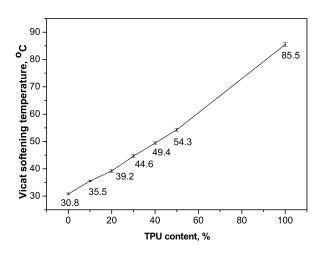
Figure 4. Effect of TPU content on Vicat softening temperatures of PPC/TPU blends.
