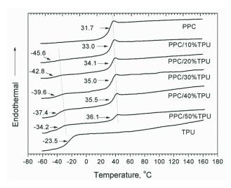
Figure 3. DSC curves of neat PPC, neat TPU and PPC/TPU blends.
