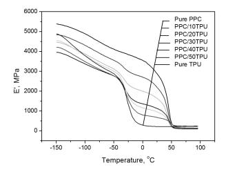
Figure 9. Storage modulus versus temperature for PPC, TPU and PPC/TPU blends.
