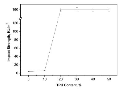
Figure 6. Impact strength of neat PPC and PPC/TPU blends as a function of TPU contents.
