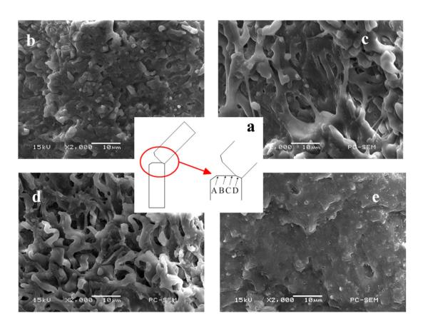
**Figure 8.** SEM micrographs of different regions on the impact fractured surface of the PPC/30%TPU sample. (**a**) Different regions of the impact fractured surface, (**b**–**e**) correspond to A–D in a, respectively.
