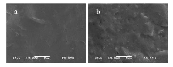
Figure 2. SEM micrographs of PPC and PPC/TPU blends. (a) Neat PPC, (b) PPC/10% TPU.
