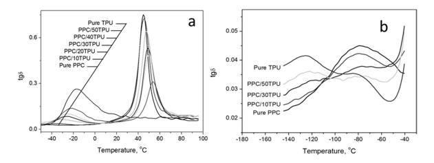
**Figure 10.** tg  $\delta$  versus temperature for PPC, TPU and PPC/TPU blends: (a) higher temperature, (b) lower temperature.
