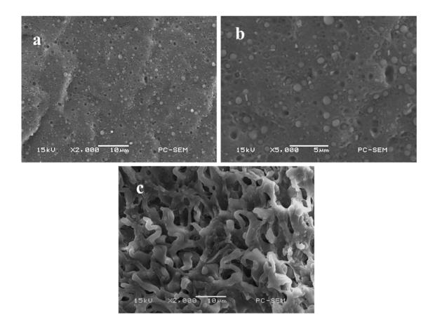
**Figure 7.** SEM micrographs of the impact fractured surfaces of PPC/TPU blends: (**a**) PPC/10%TPU, (**b**) enlarge view of a, (**c**) PPC/30%TPU.
