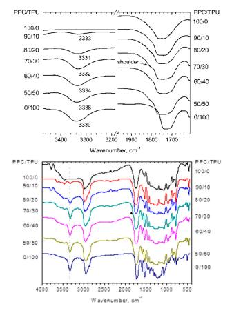
Figure 1. FTIR spectra of neat PPC, neat TPU and PPC/TPU blends.
