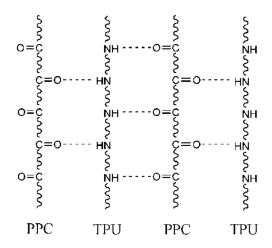
Scheme 1. Schematic illustration of hydrogen-bonding between the molecules of PPC and TPU.
