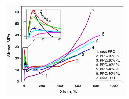
Figure 5. Stress-strain curves of PPC/TPU blends with different TPU contents.
