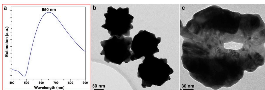
**Figure 1.** (a) UV-vis spectrum of hollow-channel gold nanoflowers (HAuNFs) synthesized with ascorbic acid (AA). (b) TEM image showing multiple branches on the outer surface; (c) TEM image in an orientation showing the hollow channel in the center.
