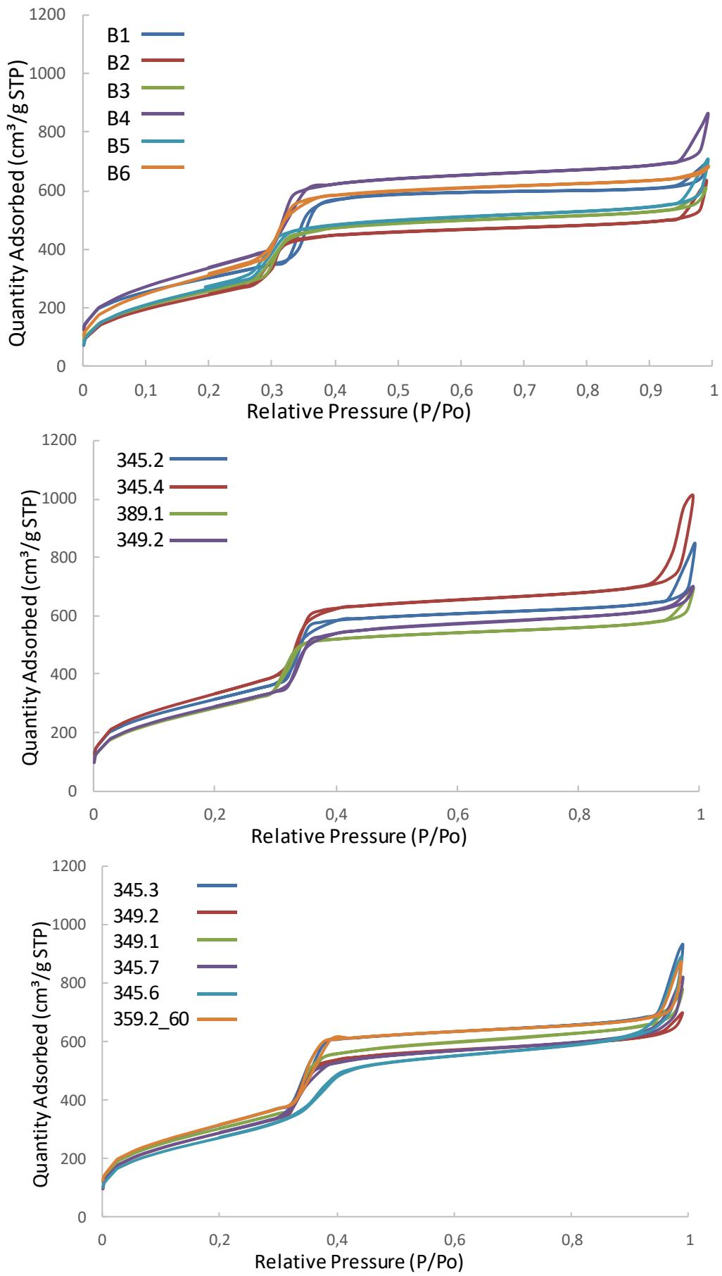
Pore diameters obtained from by N<sub>2</sub> adsorption isotherms of prepared MCM-41 MSNs.
