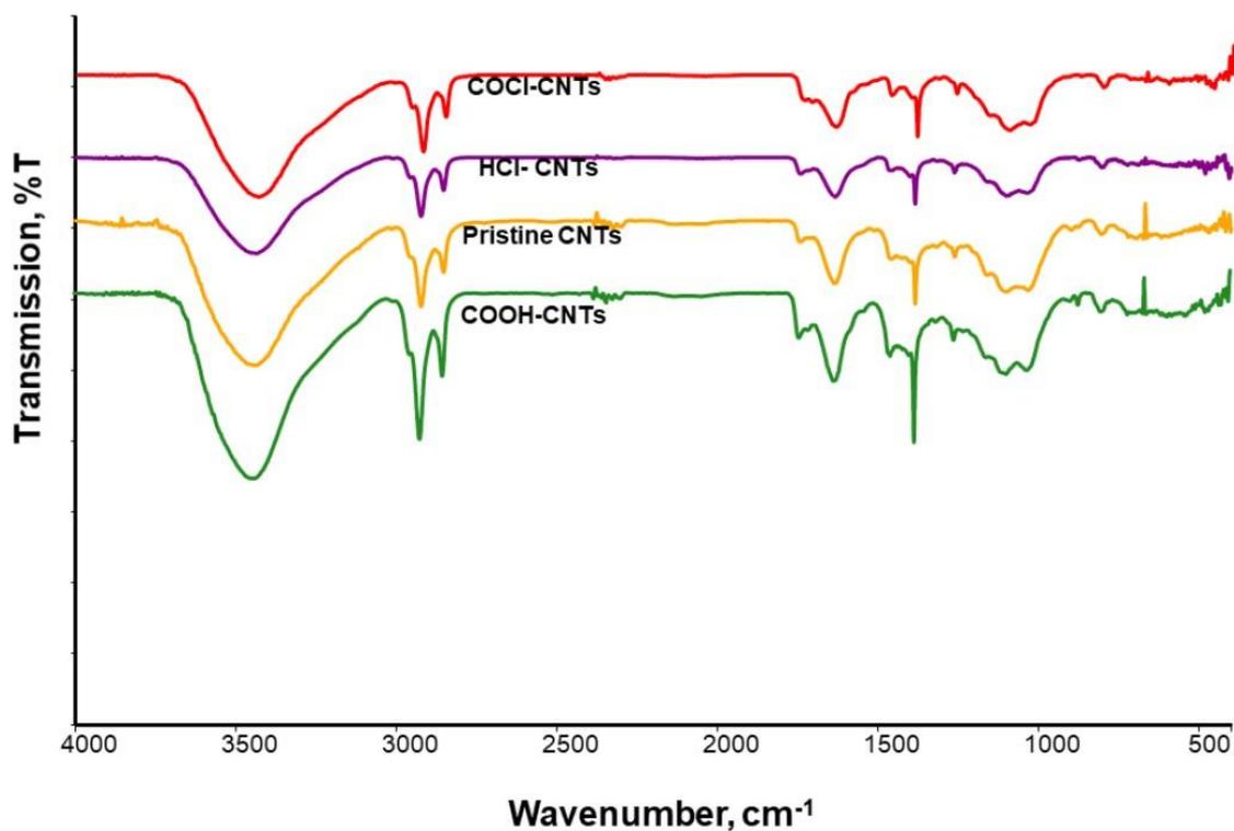
**Figure S1.** IR spectra of functionalised MWCNTs collected from KBr pellets.
