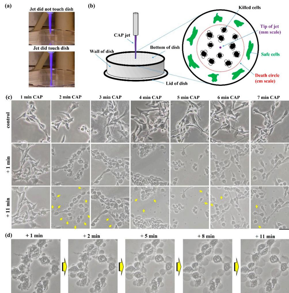
**Figure 1.** Cell death in physically based CAP treatment: (a) Photos of the CAP jet's tip; (b) schematic illustration of microscopic observation on physically triggered cell death. The damaged area by physical effect is much larger than the size of the CAP jet's tip. All microscopic observations focused
