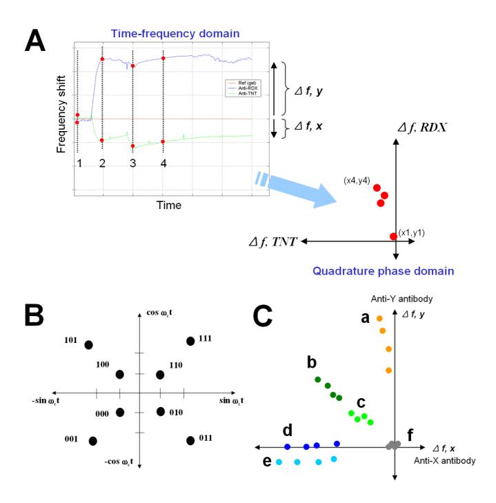
**Figure 3. (A)** Conversion from time-frequency domain to the quadrature phase domain. **(B)** 8-ary QAM constellation diagram. **(C)** two channel immunosensor signal state-space map
