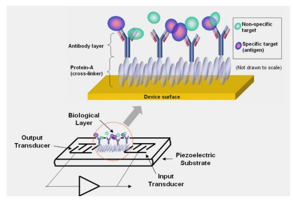
Figure 1. Schematic of a SAW immunosensor
