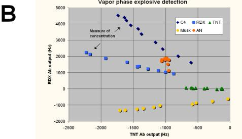
Figure 4. Explosive substances and analogues used for the experiments (A), and the signal state-space map of explosive samples (B).
