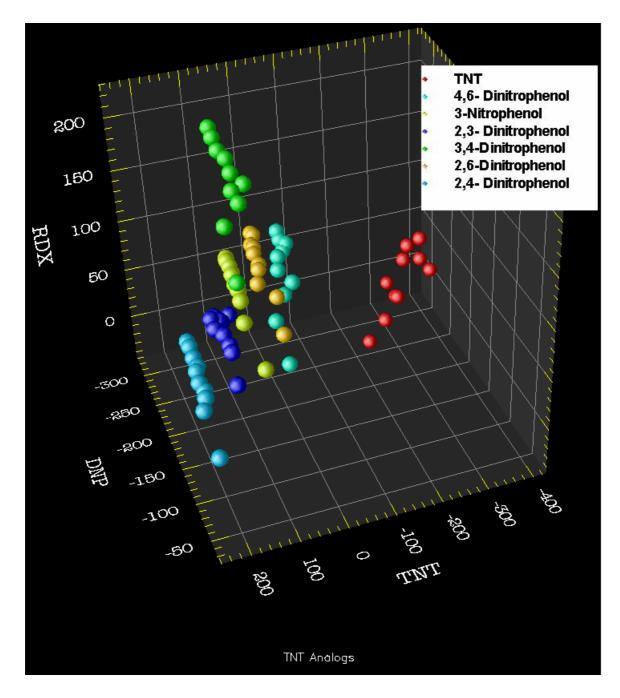
**Figure 5.** A three dimensional signal state-space map generated from the signature of three channel semi-orthogonal immunosensors system. Each individual sensor is coated with anti-TNT, anti-RDX, and anti-DNP antibodies respectively. The headspace vapor of various soil samples containing TNT and nitrophenol analogues were analyzed.
