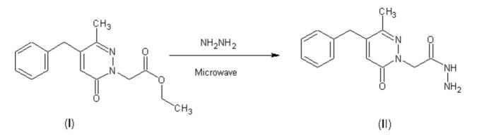
To (0.86 g, 3 mmol) of ethyl (4-benzyl-3-methyl-6-oxopyridazin-1(6H)-yl)acetate (I), was added 10 ml of hydrazine hydrate. The mixture was placed in a pyrex tube which was then introduced into a Maxidigest MX 350 Prolabo microwave [4] monomode reactor and refluxed for 10 min on 60 w as irradiation power. After cooling, the product precipitates, and then is recrystallised in absolute ethanol, yield: 85 % of (II) solid.
