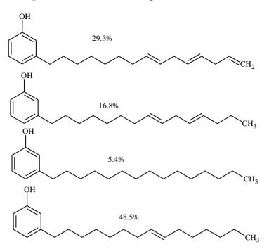
Figure 1. Structure and composition of cardanol.
