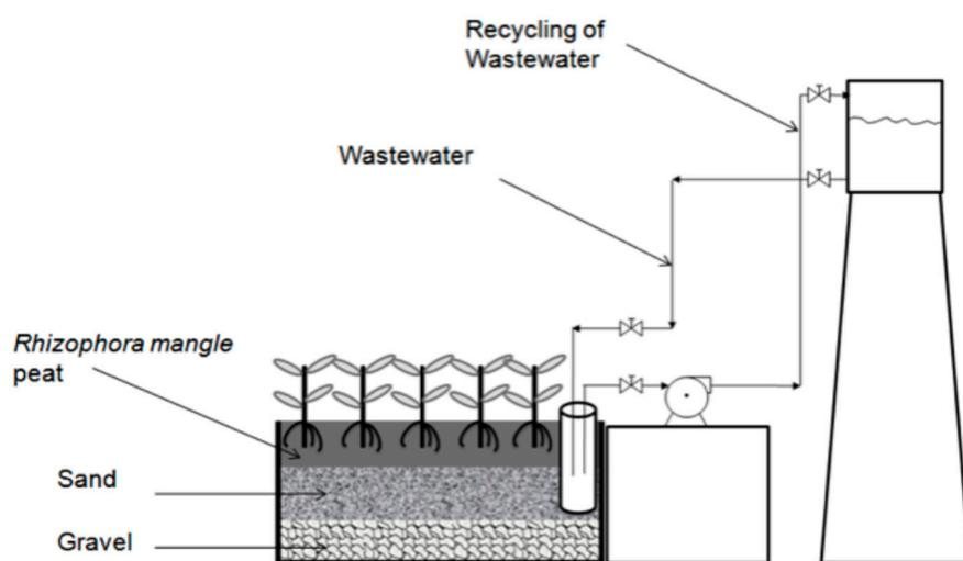
**Figure 1.** Diagram of the treatment system on secondary urban residual waste waters with subsurface recirculation.
