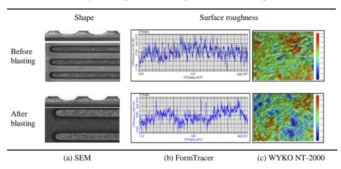
Figure 3. Shape and surface roughness of the etched sample.
