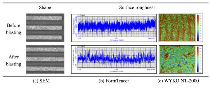
Figure 4. Shape and surface roughness of a sample that was fabricated by endmilling.
