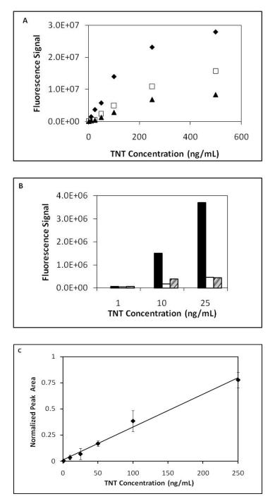
Further immunoassays were performed to test antibody specificity. Results showed that RDX, HMX and 4-nitrotoluene (4-NT) had minimal to no crossreactivity with the TNT antibody. Sensor response, as shown in Table 1, for the non-aromatic molecules (RDX and HMX) and 4-NT resulted in <3% crossreactivity. However, 2,4-DNT and 2-amino-4,6-DNT produced slightly higher fluorescence single responses with crossreactivity for 2,4-DNT and 2-amino-4,6-DNT at 24.8% and
