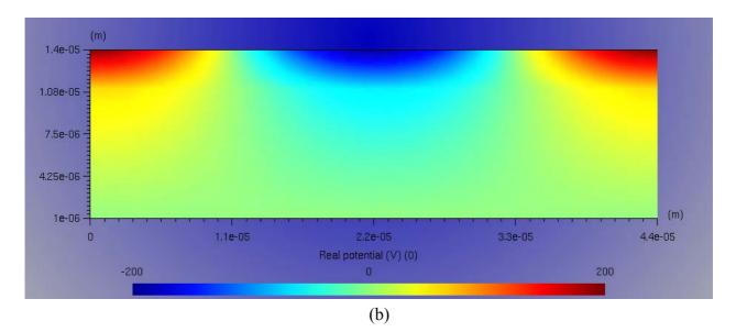
Figure 5 represents the potential at the interface *versus* the conductivity. Typical maximum discrepancies are lower than 0.1%.
