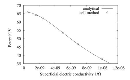
We have also calculated the electric field at the interface. CM results and analytical solution results are illustrated in Table 4 and Figure 6 for a superficial conductivity of  $1/(600 \cdot 10^6) 1/\Omega$ . The error between the results obtained using analytical equations and the CM is neglected.
