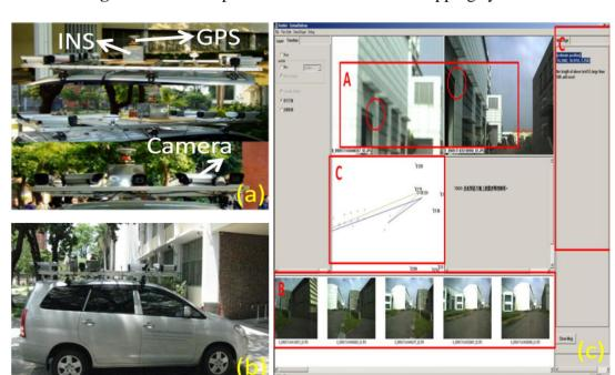
**Figure 1.** An example of a land based mobile mapping system.
