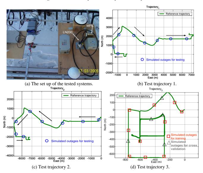
Figure 17. The tested systems and experimental trajectories.
