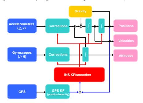
**Figure 3.** A loosely coupled INS/GPS integration architecture (closed loop).
