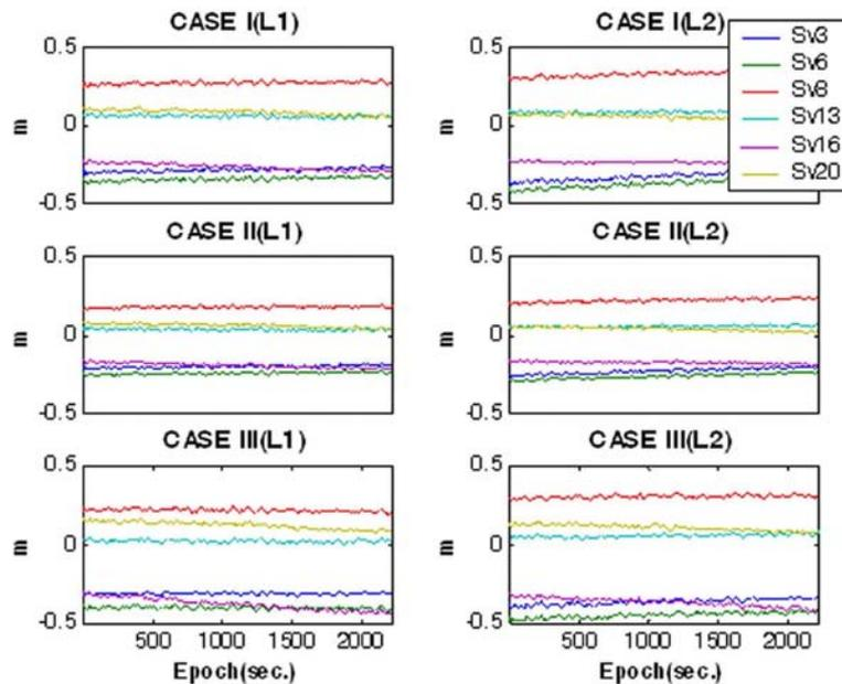
**Figure 8.** DD residuals of mobile receivers. (a) Single-reference station mode. (b) Multiple-reference stations mode.
