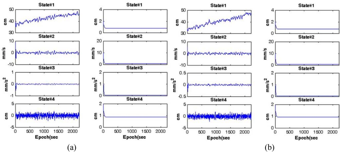
**Figure 6.** Impact of Kalman filtering in the estimation of the GPS baseline-dependent errors of SV8(CASE I).
