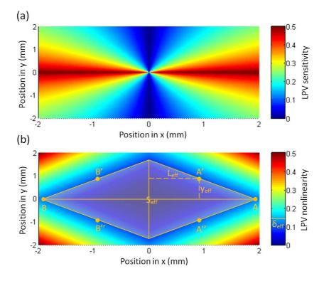
Equation (29) indicates, to keep the nonlinearity within an acceptable range, any increase in the vertical offset distance should be compensated by the decrease in the effective contacts' distance. Therefore, we can define an effective linear area (in the surface of the device), within which the LPV nonlinearity is less than the acceptable value of  $\delta_{eff}$ . According to Equation (29), this effective linear area [see Figure 20(b)] can be calculated as:
