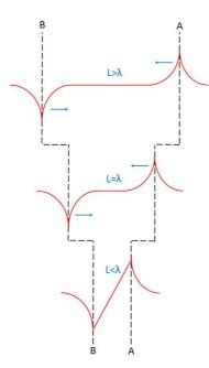
Figure 19 gives a simple picture regarding the contacts' distance effect. When two contacts' distance is very large (compared with the diffusion length), electron density at one contact (which
