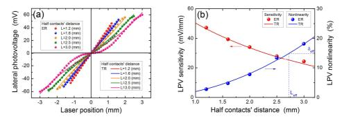
Figure 9(b) shows the increase in the contacts' distance will decrease the LPV sensitivity. For example, when the contacts' distance is at 2.4 mm, the LPV sensitivity can obtain a large value of 47.2 mV/mm, but when the contacts' distance is extended to 6.0 mm, the LPV sensitivity will be decreased to a small value of 24.3 mV/mm. Therefore, a smaller contacts' distance can not only achieve a larger LPV sensitivity but also obtain a higher linearity.
