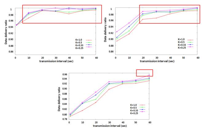
In general, the collision domain size is a major consideration to determine the effective throughput. However, since pole transformers stand in a row in our system, the power quality data is forwarded in a peer-to-peer manner except at branch nodes with more than one child node. The collision domain size is three. As shown in the figure, the effective throughput is acceptable for providing the desired power quality monitoring service.
