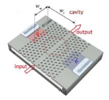
The PhC nanocavity is characterized by an intrinsic Q factor of  $8.4 \times 10^5$ . This high Q value permits the obtention of a high generation of photocurrent into the cavity region, enabling the possibility of detecting even low input power. In particular, an external quantum responsivity of 16 mA/W at a resonance wavelength of aproximately 1,500 nm, has been measured. Furthermore, on the one hand,
