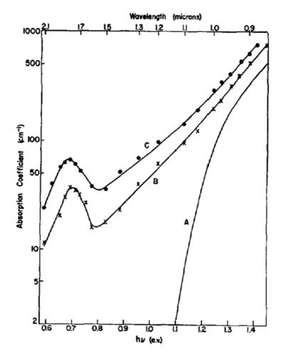
Starting from these results, many authors have induced mid-bandgap energy levels via defect incorporation into the silicon lattice by Si<sup>+</sup> ion implantation. For this material system, two typologies of crystal defects are believed responsible for sub-bandgap radiation absorption: divacancies and interstitial clusters [23].
