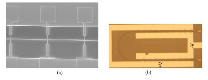
Small conductions arms intersects the waveguide defining the active regions of the photodetector. The waveguide was developed with a cross section of 500 nm  $\times$  100 nm in order to increase overlap
