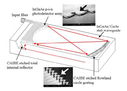
A TIR mirror was utilized to couple the optical signal from the waveguide into the detector. The typical waveguide photodetector utilizes the optical waveguide to fan out for signal detection. To avoid optical channel cross talk, the distance between the waveguides is usually  $30-50 \mu m$ , which limits the resolution. Our receiver module detector array was designed to be placed onto the Rowland focus circle to increase the detector resolution for dense WDM applications.
