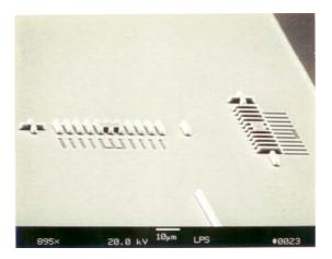
Figure 6. Verniers for different layer alignments [21].
