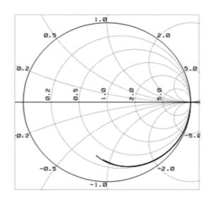
Figure 11. Smith chart for the monolithically integrated photodetector.
