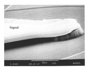
Figure 9. 10-µm diameter photodetector with coplanar metal waveguide.
