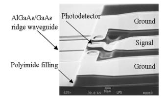
Figure 10. Reflectively coupled waveguide photodetector with metal coplanar waveguide [22].
