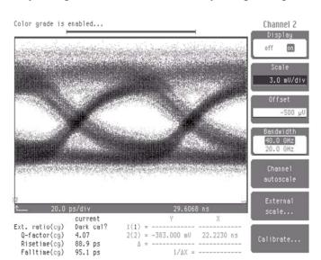
Figure 13. Eye diagram of the monolithically integrated photodetector.
