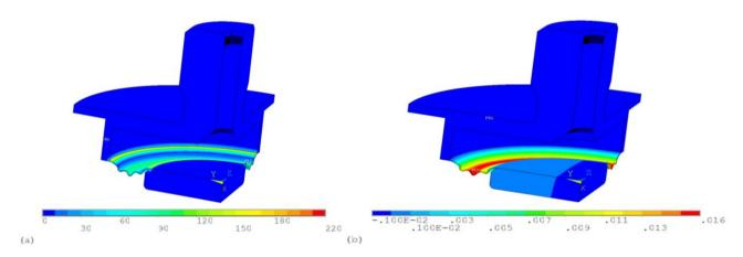
The detailed stress analysis of optical fiber deformation was made for the calculation of cross deformation, which is used for pressure evaluation using a sensing method based on the fiber Bragg grating deformation. The symmetry of geometry was also assumed, so only one quarter of the optical fiber was modeled [Figure 4(b)]. The effect of fiber-end loading was neglected, so 2D analysis was assumed.
