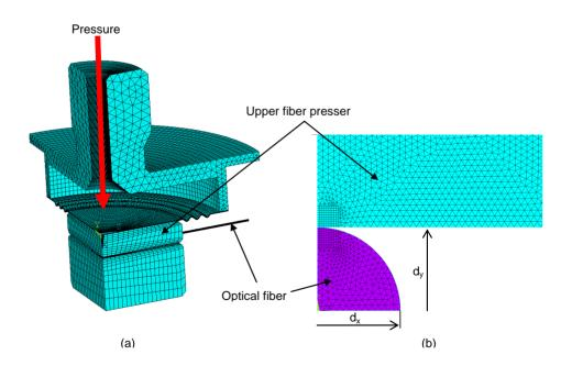
The ANSYS software, which comes from the finite elements method (FEM), was used for computational modeling in [34-41]. The stress analysis was divided into two computational parts. The first part is targeted to global stress analysis. The result of the first analysis was used for the second
