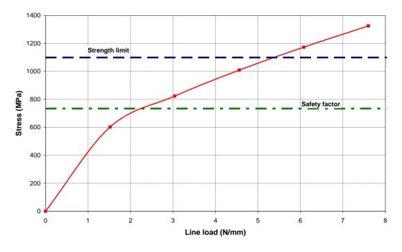
**Figure 6.** Relationship of maximal Von Mises stress in the optical fiber on an optical fiber line load with respect to a strength limit of 1,100 MPa and safety factor of 1.5.
