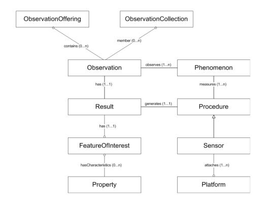
**Figure 9.** OGC Data Model for O&M.
