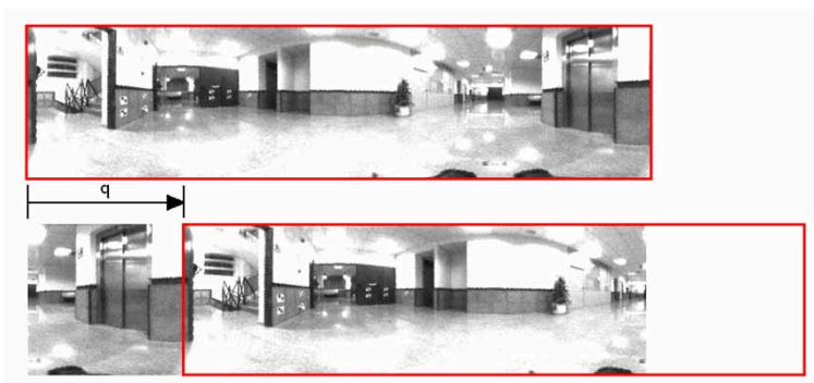
Figure 2. A robot rotation in the ground plane produces a shift in the columns of the panoramic images captured.
