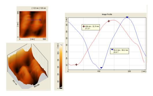
**Figure 4**. AFM image of porous Si after Pt deposition and second stage of etching. The top left figure is two dimensional image in an area of 500 nm by 500 nm and the bottom left figure is its 3D surface image, where its analysis is shown in the right figure along the arrows.
