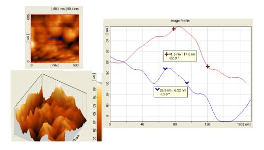
Before platinum deposition and the second etching process, thin hills with an average width of 70 nm and average height of 126 nm are seen in these pictures. After platinum deposition and the second
