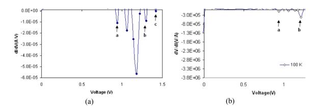
**Figure 7.** Differential conductance curve (dI/dV) as a function of voltage at 77 K (left figure). Differential resistance curve as a function of voltage at 77 K (right figure). Negative differential resistance can be seen at points a, b and c.
