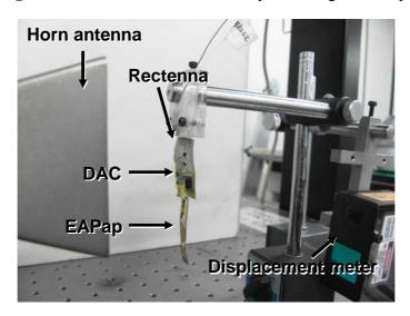
Figure 12. Microwave driven EAPap actuating test setup.
