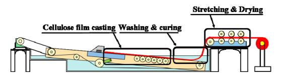
The centrifuged cellulose solution was cast on a belt using a doctor blade and cured with DI/IPA mixture, followed by the stretching/drying process. Figure 11 shows the automated process for the Piezo-paper fabrication. For curing, mist of curing solvent that consists of deionized (DI) water/Isopropyl alcohol (IPA) was sprayed. The resultant gel-like cellulose film was slowly immersed into the solvent mixture (DI/IPA) bath to effectively eliminate Li<sup>+</sup> ions as well as DMAc [18]. After
