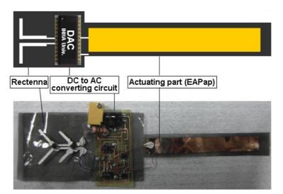
Figure 9. Configuration of Microwave driven EAPap actuator.
