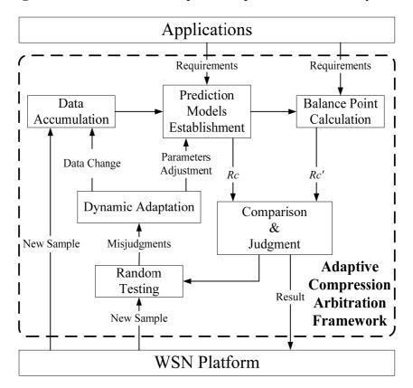
Figure 11. Framework for adaptive compression arbitration system.
