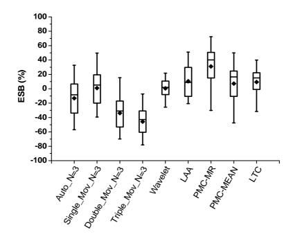
Figure 9. Compression algorithms comparison in ESB at the node level.
