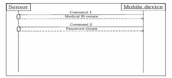
Figure 6. Protocol between mobile device and sensor.
