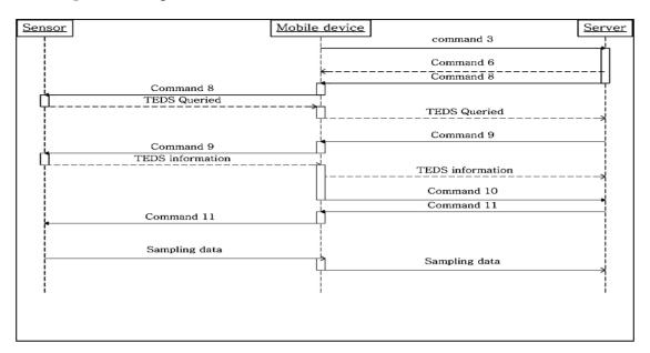
Figure 7. The protocol between the sensor, mobile device and server.
