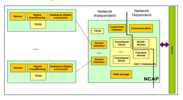
Figure 1. Sensor node and NCAP structure.
