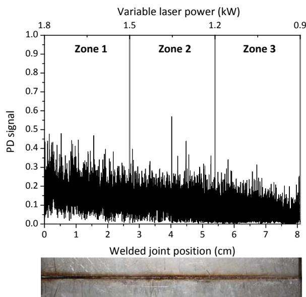
The acquired optical signal as a function of the welded joint position and of the variable laser power, together with the top picture of the joint are shown in Figure 5. The photodiode signal exhibits only a slight decrease of its mean value as far as the laser power is lowered.
