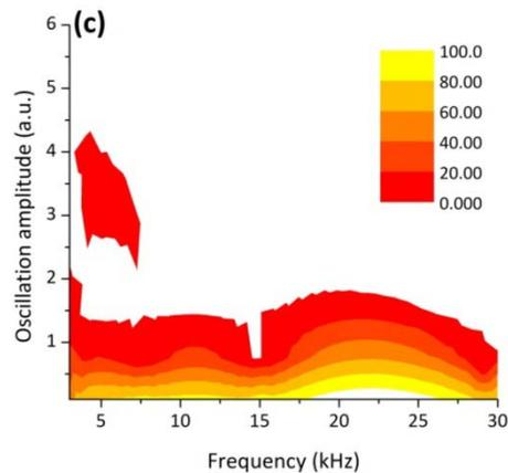
The capability of the wavelet analysis to detect variations of the welding conditions induced by changing of the main process parameters was further examined by decreasing the laser power from 1.8 kW to 0.9 kW during the run and keeping the welding speed at a constant value of 80 mm/s.
