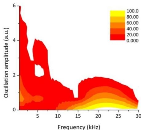
The photodiode signal depicted in Figure 2 was then divided into three zones and the DWT was calculated for each segment in order to see if any difference could be noticed on the frequency distributions thus checking the reliability of this technique. In Figure 4 the relative oscillation amplitudes as a function of the frequency bands are reported corresponding to the three different weld segments. The frequency distributions are nearly equivalent among the three graphs.
