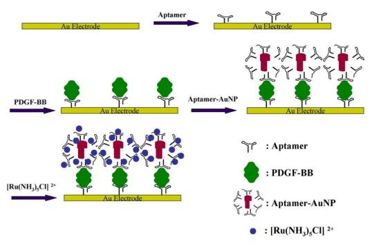
**Figure 5.** Scheme for the formation of sandwich structure and Au-NPs mediated amplification for PDGF detection (adapted from reference [21], with kind permission).
