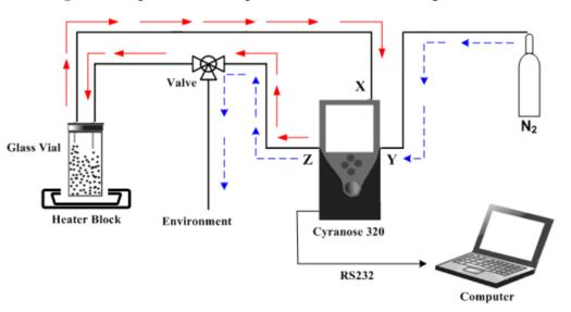
Figure 2. Experimental setup for the classification of agarwood oil.
