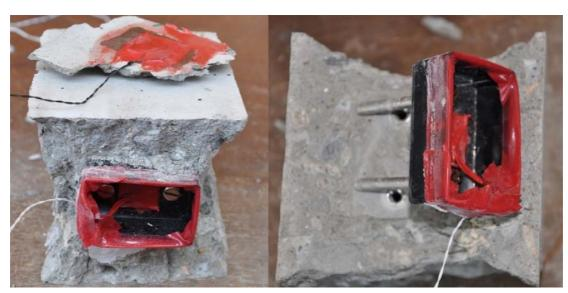
Figure 5. Reusable setup detached after compressive loading.
