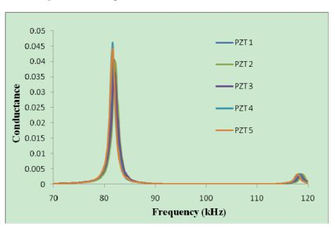
Figure 6. Free signatures obtained from PZT transducers.
