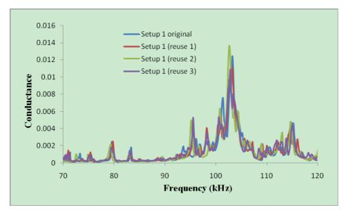
Figure 9. The initial signature obtained from setup after installing inside the concrete.
