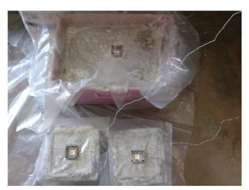
Figure 2. Monitoring hydration rate with reusable PZT transducers in Cast 4.
