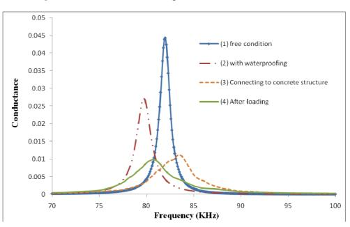
Figure 11. Variation of PZT signatures in different conditions.
