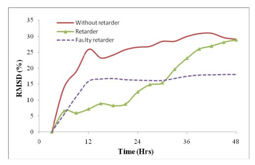
It can be seen from Figure 13 that the concrete containing retarder gains strength rather gradually, hence to safely remove the molds, the minimum curing time is around 36 hours. For the faulty retarder, the RMSD changes show that the concrete undergoes some initial changes but progresses at much slower hydration rate.
