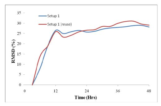
The RMSD values based on comparison between the signatures measured at different measurement points and the signature at the third hour have been calculated for each mixes. Figure 12 shows the good repeatability of RMSD values for setup 1a in Cast 1 and 2.
