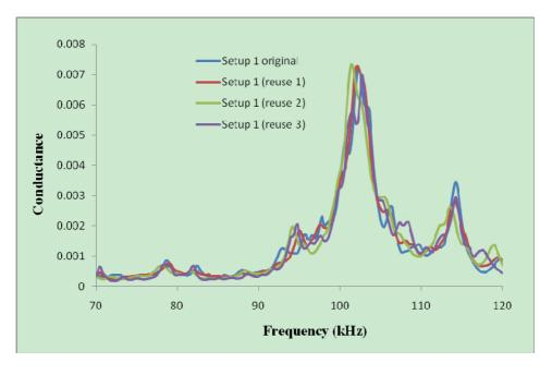
As shown in Figure 8, the process of removing the aluminum enclosure from one concrete specimen and reusing it in another specimen has a minor effect on the signatures. The repeatability of signature is very good, even if no water proofing coating was applied on this setup. For the plastic enclosure with waterproofing coating used in Casts 7 and 8, better repeatability has been obtained.
