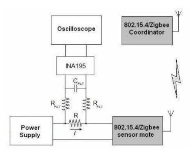
Figure 1. Experimental setup for the measurements of battery consumption.
