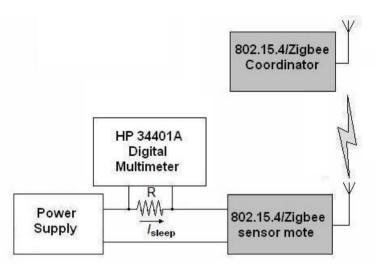
Figure 6. Experimental setup for the measurements of battery consumption during sleep mode.
