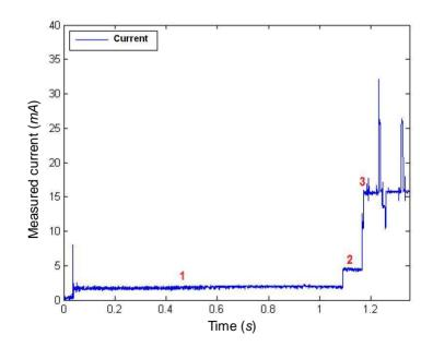
Before transmitting any data, the sensor has to detect the presence of the Coordinator and proceed to its association. The measured evolution of the required current during this operation is illustrated in Figure 3 and is composed of the following phases:
