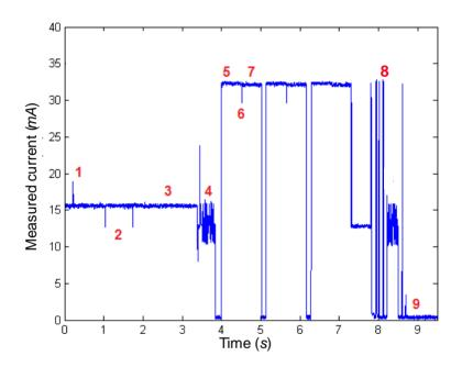
Interval 4: After the role of the mote (final device) is decided, the microcontroller sends the corresponding orders to the ZigBee processor to initiate the search for a Coordinator. After that, the microcontroller enters sleep mode (with an extremely low consumption).
