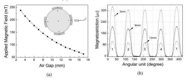
The asymmetry of the magnetic field may be noticed for the three air gaps analyzed. In the case of the 13 mm air gap, the difference between the two maxima is  $7.8 \times 10^{-6}$ , and it is still possible to measure the magnetic unbalance in spite of the proximity to the resolution limit of the dynamic FBG interrogator, which was of approximately  $5 \times 10^{-6}$ .
