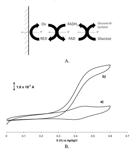
Ferrocene-derivative mediators and GluOx can be incorporated into various types of matrices that are attached to an electrode surface so that the enzyme and mediator system are confined to a small volume adjacent to the electrode surface and cannot freely diffuse throughout the solution. The advantage of having both the mediator and the enzyme confined to the surface is that a higher degree of organization can be achieved, confining the system to a small dimension restricts the electron
