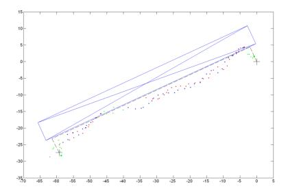
**Figure 10.** Solutions under adverse conditions (f): (i) autonomous code positioning; (ii) custom positioning procedure with C1&D1; (iii) custom positioning procedure with C1&D1, plus ionosphere and troposphere models; (iv) internal positioning of the receiver. Units are in meters.
