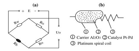
The catalytic element is electrically heated to about 400  $\,^{\circ}$ C, at which temperature catalytic oxidation of the methane readily occurs. The rise in temperature, with the corresponding increase in the resistance of black element produced by reaction on the catalyst, is then measured by incorporating the element in the Wheatstone bridge network where the potential difference across the bridge forms the output of the device, as shown below:
