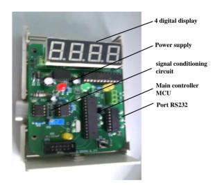
The constant temperature circuit is simply presented in Figure 9. By adjusting the current I automatically, the working temperature as well as the resistance of catalytic element  $R_b$  remain constant. The methane gas concentration can be detected by measuring the current variation  $\Delta I$  which is proportional to methane gas concentration [24,25]. In this way, the range of measurement is extended to 0–10%, and response time is shortened.
