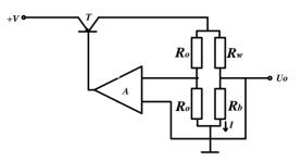
Figure 9. Measurement circuit with constant voltage.
