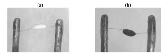
The prepared white and black elements were matched by a dynamic matching method. The best matched elements were encapsulated with epoxy resin and connected as an electrical bridge. Bridge<sub>Al</sub> stands for bridge containing Pt-Pd/Al<sub>2</sub>O<sub>3</sub> catalytic element, bridge<sub>n-Al</sub> stands for three bridge containing Pt-Pd/  $n-Al_2O_3$  catalytic element, and bridge<sub>n-Ce-Al</sub> stands for bridge containing Pt-Pd/n-Ce-Al<sub>2</sub>O<sub>3</sub> catalytic element.
