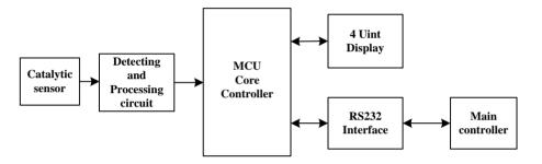
Figure 8. Signal processing module of the methane sensor.
