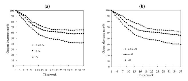
Figure 6. The stabilization comparison of three unit electrical bridges (a) 1% CH<sub>4</sub>, (b) 2% CH<sub>4</sub>.
