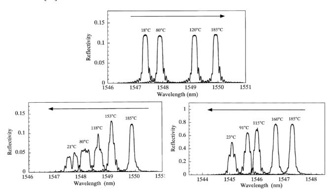
It should be clear that every type of distortion needs a different approach in determining the strain components of the structure in which the sensor is embedded. Examples of the spectral response of embedded FBGs in different FRP laminates, is shown in Figure 7. An overview of the possible methods to interpret these spectra is given in the next section.
