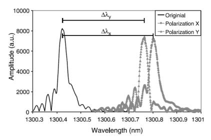
It is certain, that for *heavily distorted FBG spectra*, a simple demodulation technique such as FWHM-algorithm will not satisfy the need to quantify the global strain of a structure under load. Therefore, certain new techniques are necessary to predict the strain in a structure, and perhaps other parameters of the grating could be measured simultaneously.
