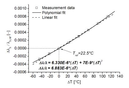
It should be apparent that any change in wavelength, associated with the action of an external perturbation to the grating, is the *sum of mechanical deformation and temperature terms*. Therefore, in sensing applications where only one perturbation is of interest, the de-convolution of temperature and strain becomes necessary! An overview of methods to decouple the temperature and strain cross sensitivity is given in Section 4, however, focus will first be on pure strain measurements.
